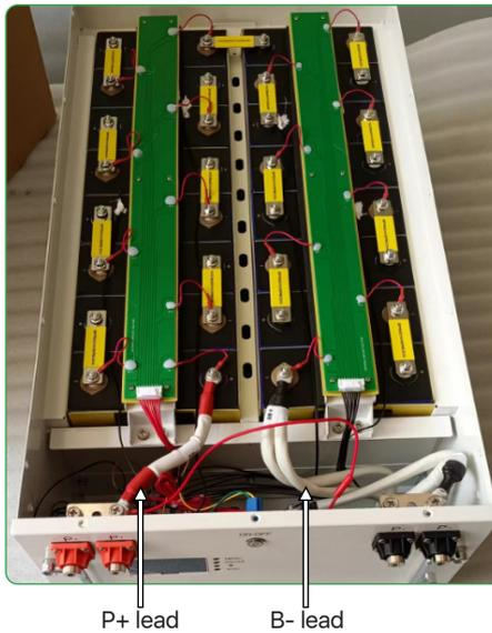
5. Check every connection, the voltage between the main positive and the negative is  $>52V$ , then turn the button on, the LCD and the indicator work out, then the assembly operation is completed, as shown in figure 5.
