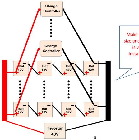
Make sure all wires are same size and length. Wire resistance is very important when installing parallel units and battery banks
